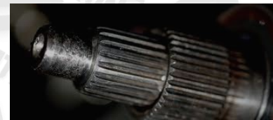
Fig 1: Splines on the input shaft
